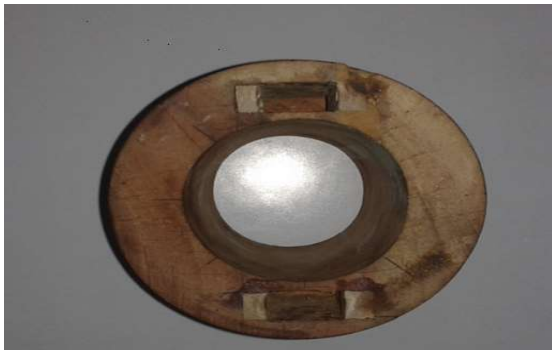
Fig.22 Fabricated Hollow Rotor of Dual Stator Machine
