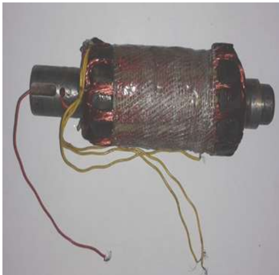
Fig.23 Fabricated Inner Stator of Dual Stator Machine
