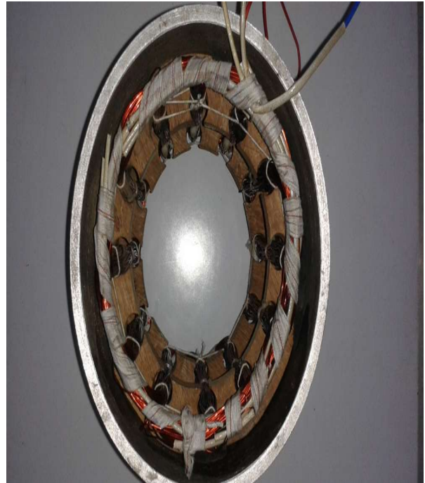
Fig.24.Fabricated Outer Stator of Dual Stator Machine
