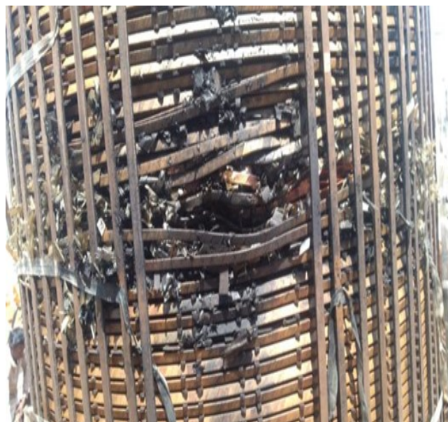
Fig. 15. Buckled tertiary winding with turn to turn short
