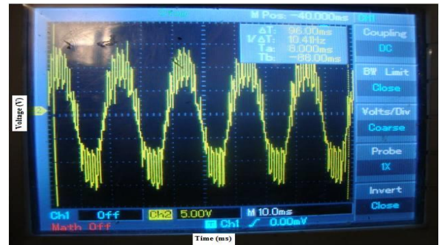
Fig.16 Distorted Load Voltage waveform due to Swell and Harmonics
