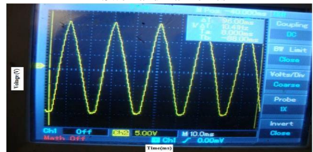
Fig.17 Load voltage get normalized when DVR activated
