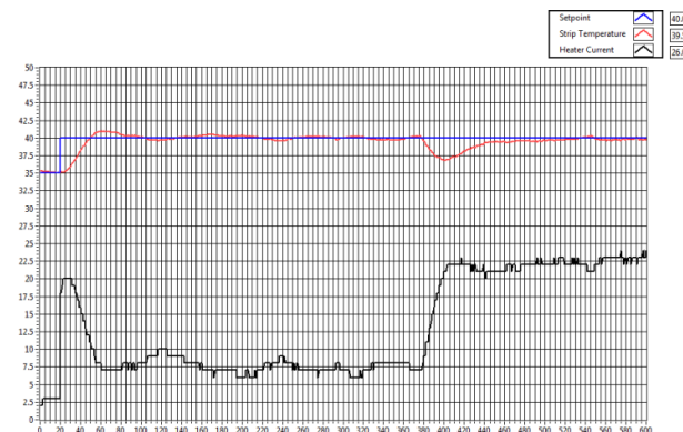
Fig. 8. PI controller closed loop response using backward difference
