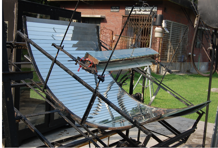
Figure 5: Cylindrical parabolic concentrator with flat horizontal absorber mounted with modified grid finger solar cells
