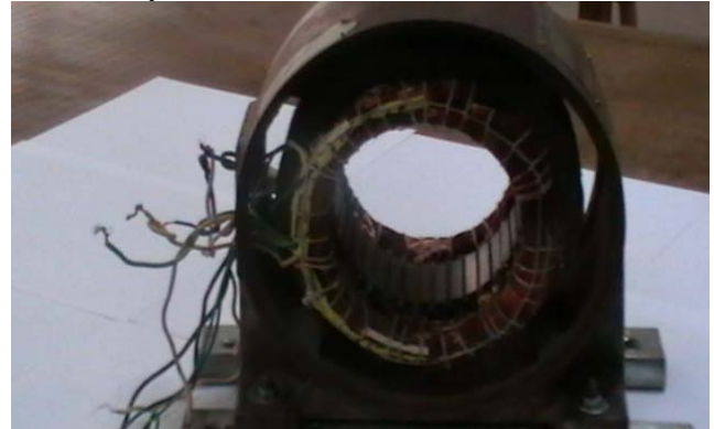
Experimental Stator of the Dual Stator Winding Mixed Pole Machine
