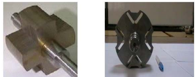
Salient Pole and Flux Barrier Rotors
