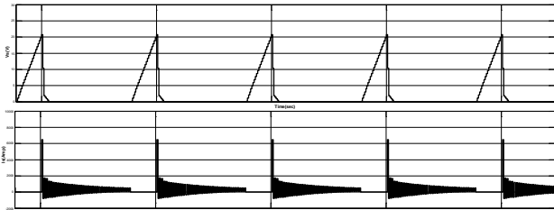
Fig.32 a)Switch Current b)Switch voltage for flyback converter in reverse mode.
