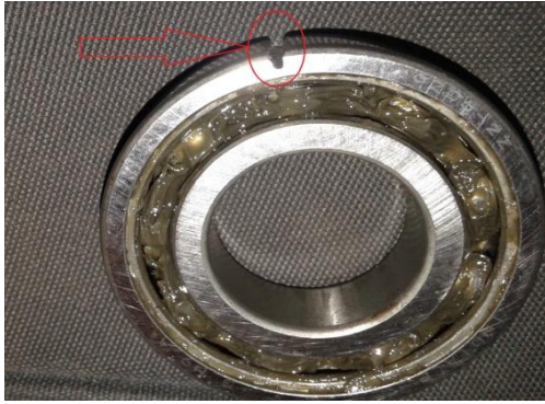
Fig.6. Bearing with outer race fault
