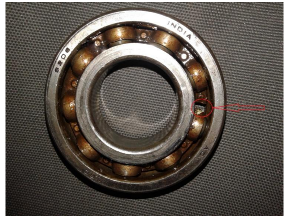
Fig.5. Bearing with cage fault
