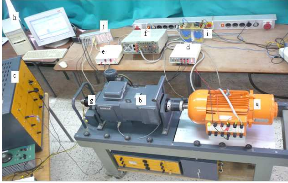
Fig. 10. Photo of the experimental system: (a: induction motor, (b,c) : system of load, (d,e): current and voltage transducers, f : IGBT based-inverter, g : incremental coder, h : PC including dSPACE, i: three-phase rectifier and capacitive filter, j: dSPACE external panel).
