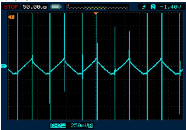
Fig. 10 Inductor current waveform corresponding C_{in}= 1000\mu\text{F} , L= 2\text{mH} , C_o=200\mu\text{F} and R_o=400\Omega and F_s=20\text{ kHz}
