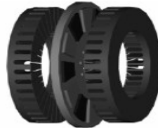
Fig. 5. Axial flux PMG with double stator
