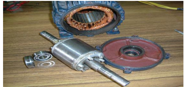
Fig 4. Parts of motor machined for implementing air gap eccentricity
