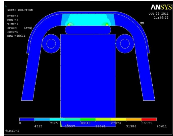
Fig. 7. Electric field pattern corresponding to Fig.6
