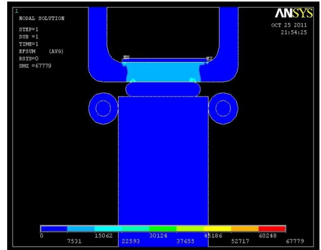
Fig. 3. Electric Field pattern corresponding to Fig. 2
