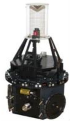
Figure 2: Swedish Wheeled omnidirectional WMR
