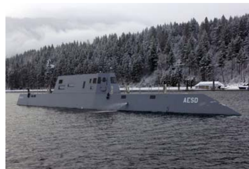
Fig. 7. Water jet propelled Destroyer model.
