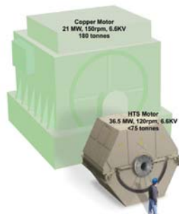
Fig. 14. Classical Motor of 21 MW 180 tonnes compared with a HTMS 36.5 MW 75 tonnes.
