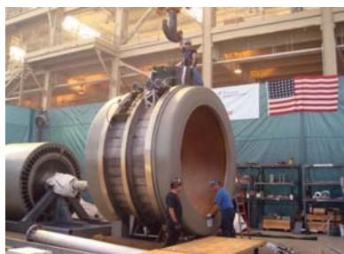
Fig. 15. Stator and rotor of 36.5MW HTSM motor.
