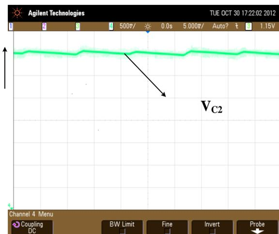
Fig.15 Experimental capacitor  $C_2$  voltage profile for  $M_a=0.9$
