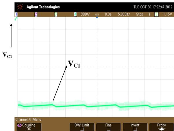
Fig.14 Experimental capacitor  $C_1$  voltage profile for  $M_a=0.9$
