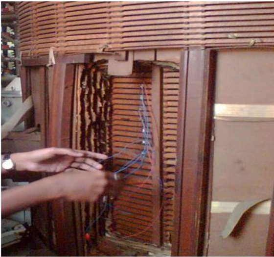
Figure 3: Shorting of discs in HV winding.
