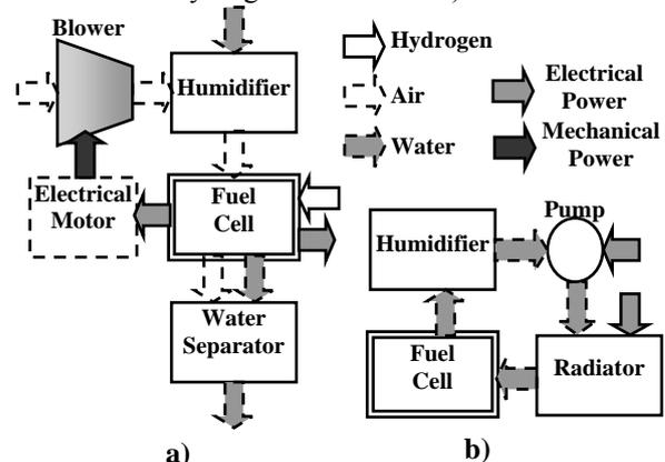
Fig.1. Fuel cell system diagram:
