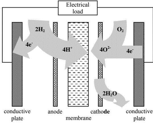
Fig.2. Basic PEFC operation.
