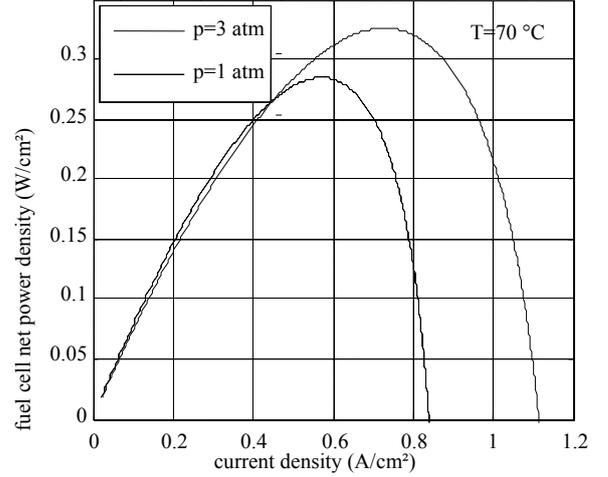
Fig.3. Fuel cell net power density for two different air pressures:
