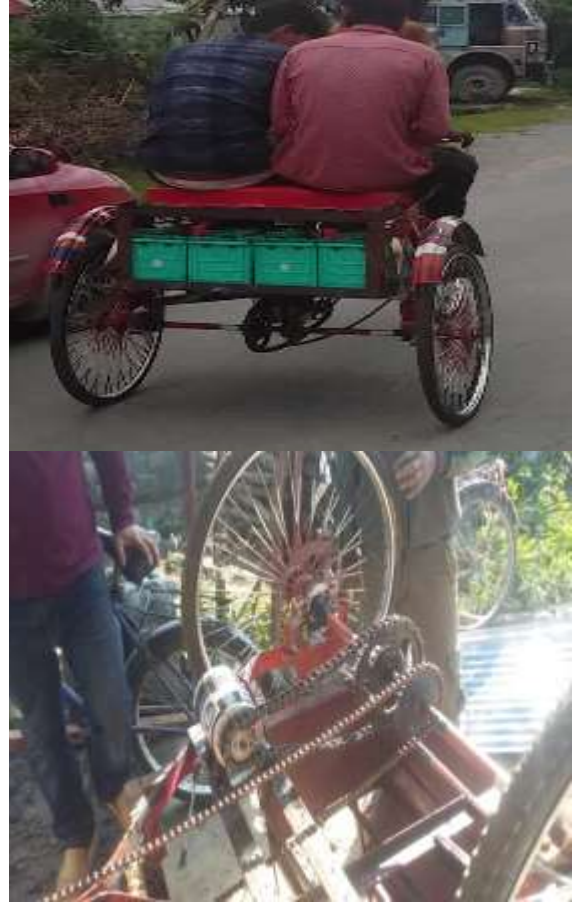
Figure 15 Mechanical assembly of modified Rickshaw
