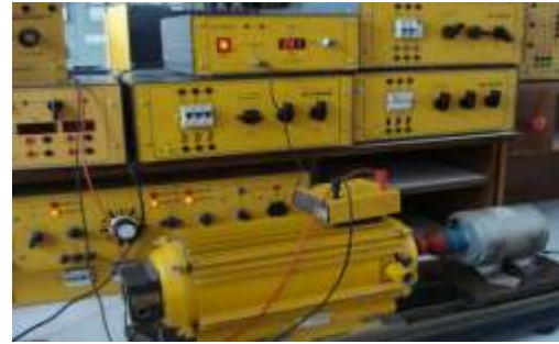
Figure 10 Experimental Setup for acquiring motor characteristics.
