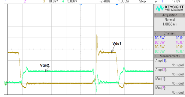
Figure 23. Synchronous switch voltage V_{ds2} and gating signal V_{gs2} ( V_{in} :45V and I_{load} :10A).
