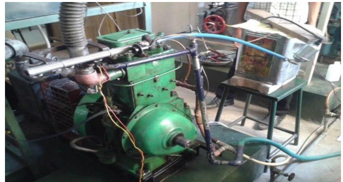
Fig 2. Engine Hardware setup for ethanol fumigation
