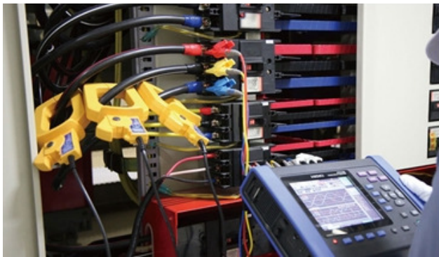
Fig. 3. Power Quality Monitoring at Feeder-1
