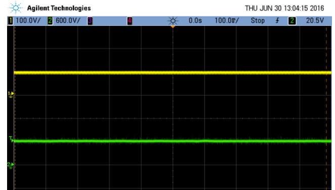
Fig.20. Input and output voltage of the boost converter
