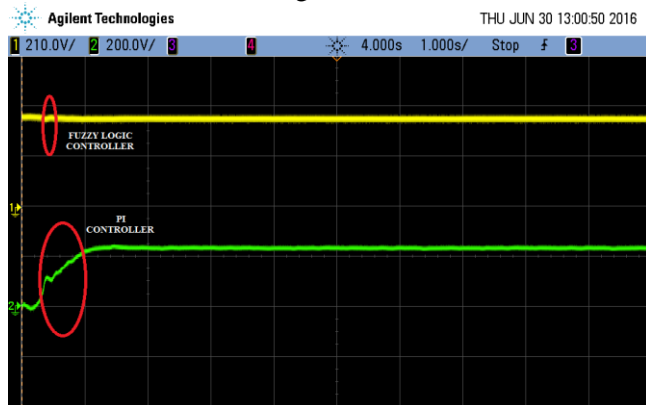
Fig.19. Transient Response of buck converter using PI and
