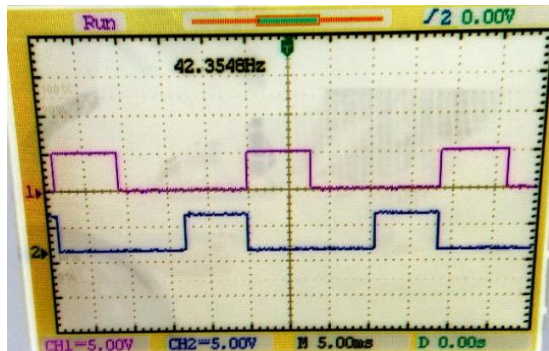
Fig. 5.5 Switching pulses applied to three-phased inverter switches of S_1 & S_3
