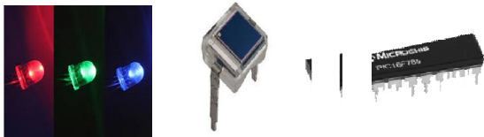
(RGB + NIR) leds BPW34 photodiode PIC16F785
