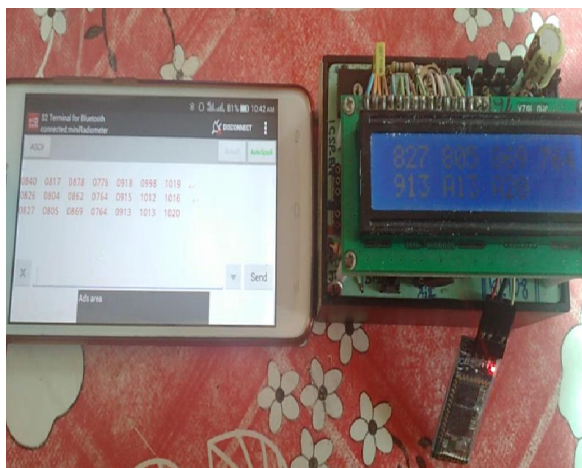
Fig.11. A preview of the miniradiometer prototype, using an optional low cost BlueTooth module, to monitor the acquisition data through an Android device.
