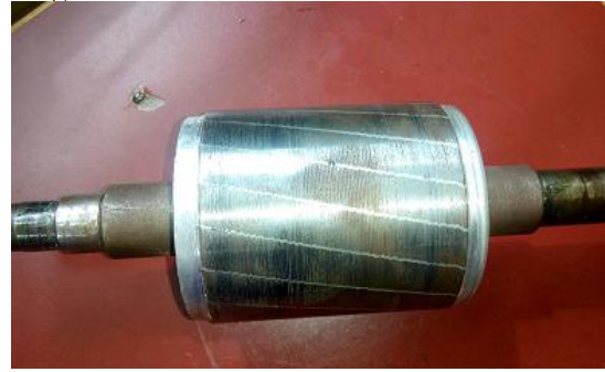
Fig3. Broken bar in the rotor
