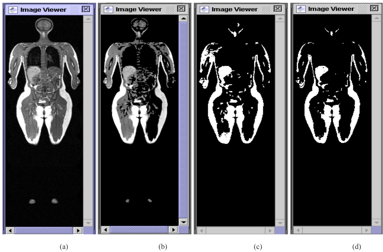
Fig. 4. Experimental data –dataset 2 (slice 26). (a) Input image. (b) Pre-processed image. (c) Image resulting after clustering. (d) Image resulting after image refinements is applied.
