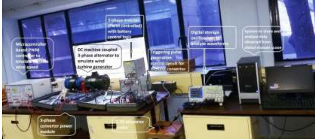
Fig. 16. Experimental module developed in the laboratory to emulate variable speed WTG to analyze power quality issues
