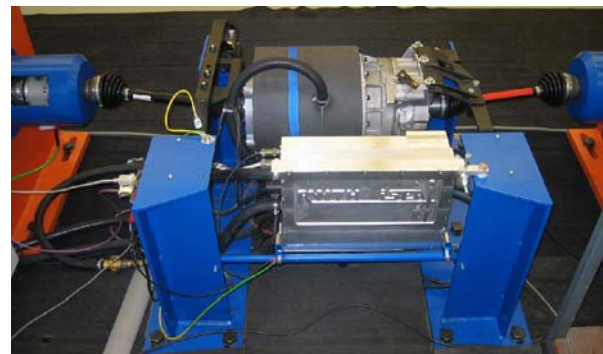
Figure 14. Test set-up showing mounting details of the propulsion unit.
