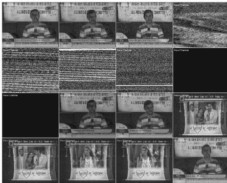
Fig. 2: Picture distortion due to antenna rotation.
