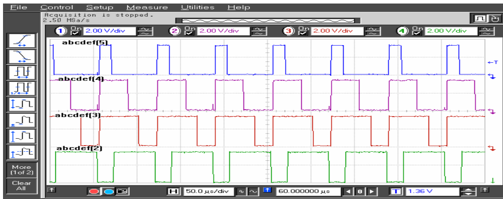
Fig. 8 Experimental testing: the oscilloscope waveforms of the first 4 PWM channels
