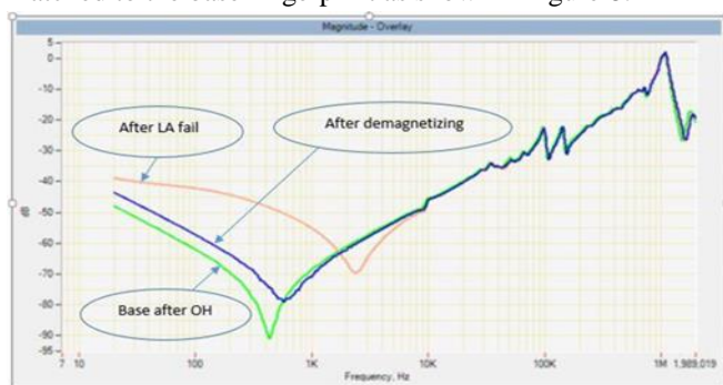
Fig. 8. SFRA of H.V. winding after demagnetization
