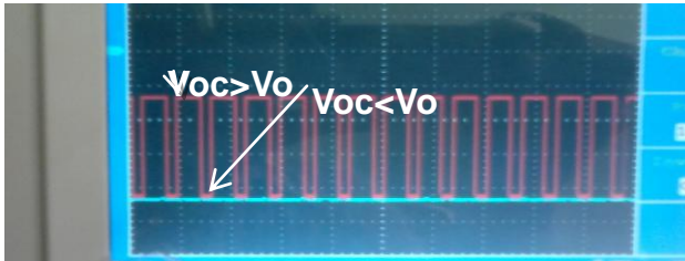
Fig 13a. Pulses generated by PIC16F877A for SMC
