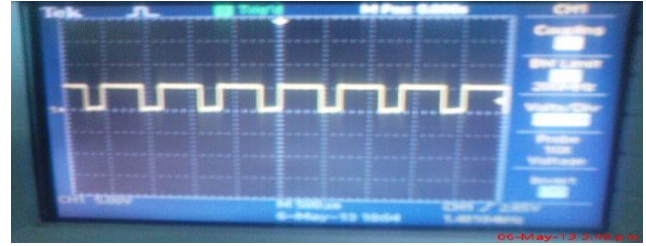
Fig 13b. Pulses generated by PIC16F877A for FLC
