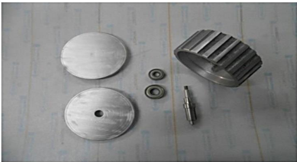
Fig. 20. Parts of the slot-less motor after machining
