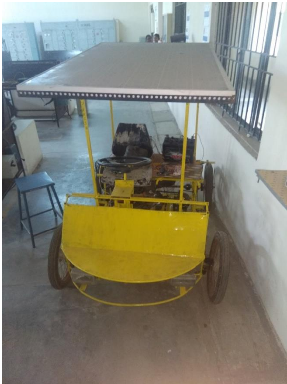
Fig. 10. Experimental setup of solar powered Brushless DC motor
