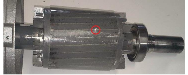
Fig. 6. Incipient outer cage bar fault
