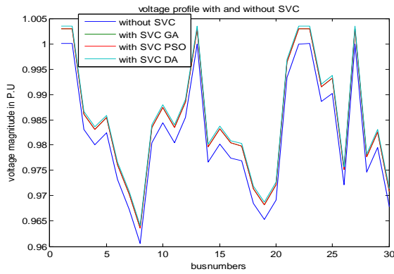
Fig. 10. Voltage profile of IEEE 30 bus with and without two SVCs
