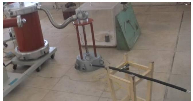
Figure 4. Specimen connected with Marx circuit
