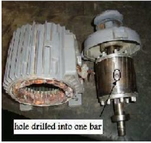
Fig.2 Seeded broken rotor bar fault.
