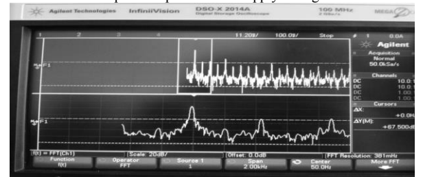
Fig. 10. Stator current spectrum for motor operating under variable load condition in Agilent DSOX-2014A with broken rotor bars
