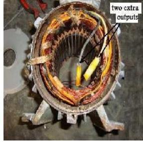
Fig.3. Seeded short-circuited windings in one stator phase.
