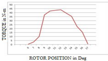
Fig. 4 Torque Vs Rotor Position Curve
