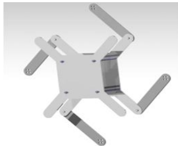
Fig 3: Design of Folded frame of Hybrid Vehicle (90degree)
