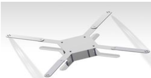
Fig 1: Design of Unfolded frame of Hybrid Vehicle (0degree)
