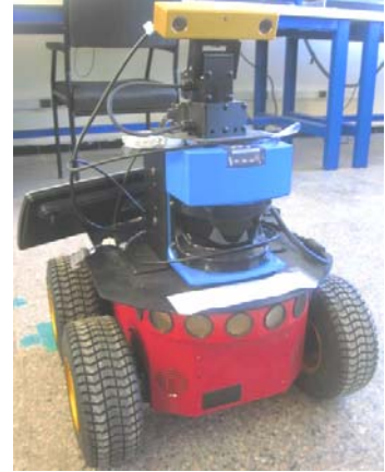
Fig 10 Pioneer 3AT mobile robot used in our Experimentations.
