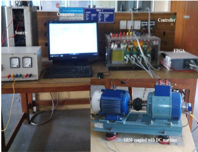
Fig. 12. Experimental Set-up for control of SRM.
