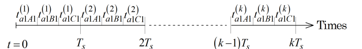
Fig. 6. Segmentation of the axis time for the consecutive orders of intervals closing of the switches.
