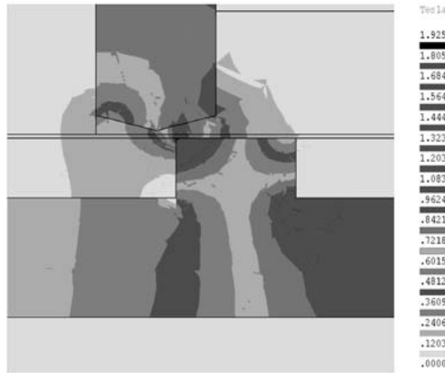
Figure 8: Flux density distribution detail for Case C.
