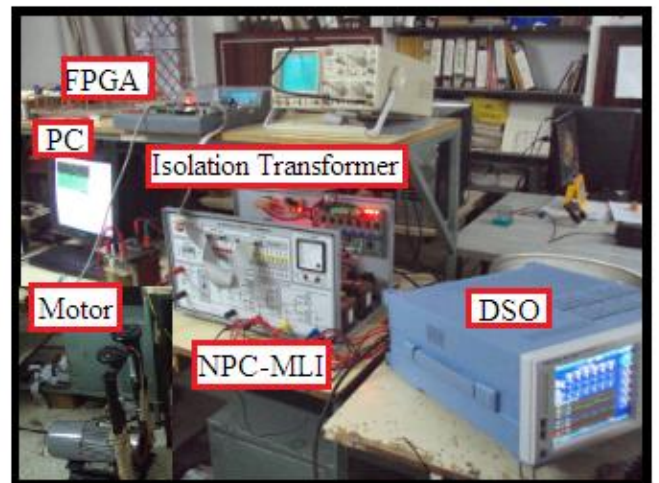
Fig.8 Experimental setup- 1kW three-phase NPC-MLI fed IM
