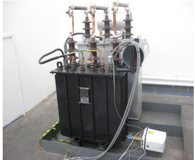
Fig.4. Measured transformer 30 kVA (black) and its power supply transformers (silver) in the laboratory.
