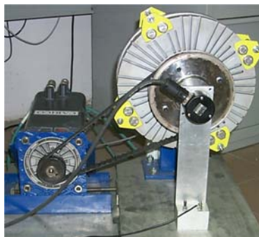
Fig. 9-b. Electrical machines in the test bench.
