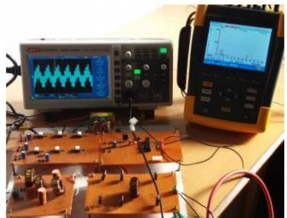
Fig.11.shows the experimental setup of the three-phase VSI connected RL load
