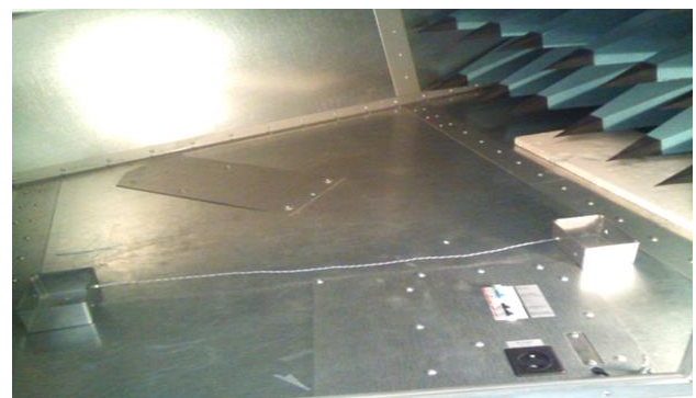
Fig. 10. Photography for experiment of a simple conductor wire inside the GTEM cell at the test zone
