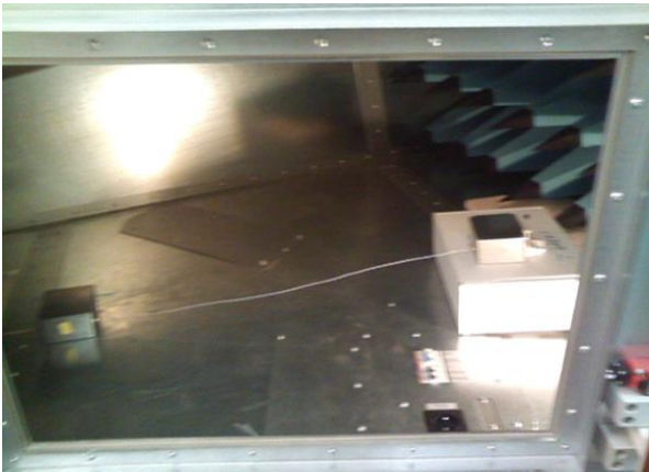
Fig. 12. Photography for experiment of a simple cable without ground
