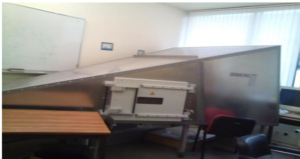
Fig. 7. Photography of the GTEM cell used in the experiment
