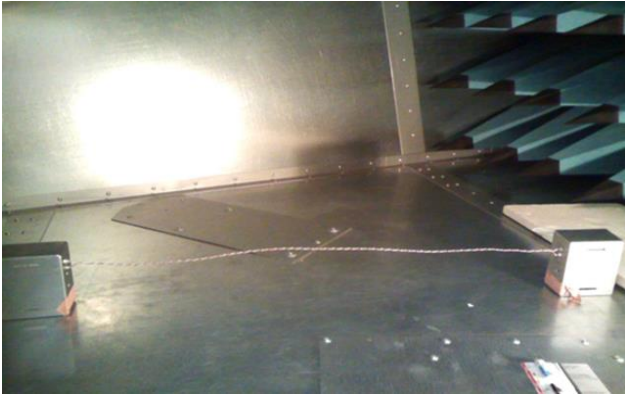
Fig. 11. Photography for the experiment of a twisted cable with height h=9\text{cm}
